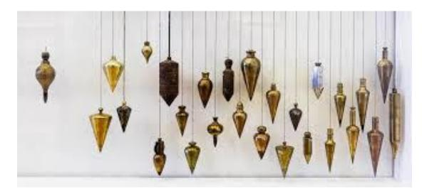
The plummet is more accurate a measuring tool than any other leveling device available, including the fancy laser levels we nerd out over, and it is the perfect metaphor for this situation. A plumb bob <u>never</u> lies. It always settles and aligns at the bottom to precisely the same location that it is at the top of a thing. That's the meaning of plumb – the bottom and top of a thing are aligned vertically. A plumb line helps you find that perfect alignment when you use it to measure.
